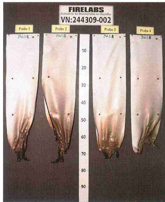
fig. 4 Photo of test specimen after the test
